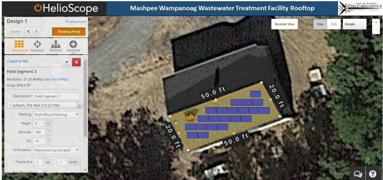
Figure 2. Potential solar development on WWTF roof. The roof face south-southeast and has a small amount of area for solar PV.
